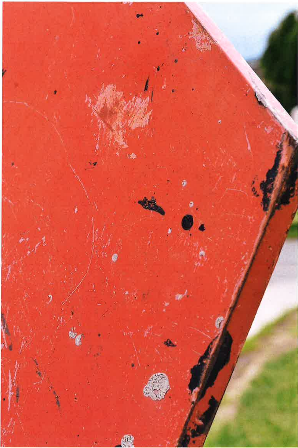
accretions, paint loss, scratches; abrasions
